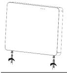
Use Philips screwdriver to unscrew the 2 holding screws located at the bottom of the panel
