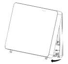
Remove the front cover of the panel by tilt it outside
